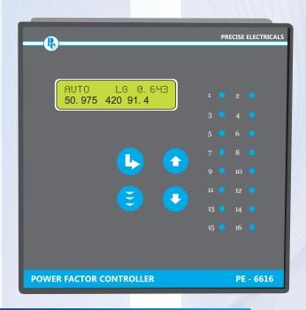
This version of 66 XX series displays all parameters such as power factor, shortfall K VAR Excess KVAR, voltage, current and T HD all at a tine. By selection, it displays % harmonic from 3rd to 13th and capacitor values. It has built in facility to cut-off the capacitors in case of harmonic overload. It has password protected settings. It's built-in TEST mode enables to test the panel without CT current. Auto as well as Manual mode of operation are available in this relay.
