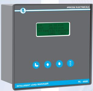
The intelligent load manager ILM 4600 is used to protect the overshoot of demand from the sanctioned demand. It facilitates controlling of up to three independent loads by continuously monitoring the demand. It has RS 485 serial port with MODBUS RTU/ASCII protocol to communicate with PC thereby providing an ideal source for effective energy management. Apart from this the user can also check various parameters simultaneously.
